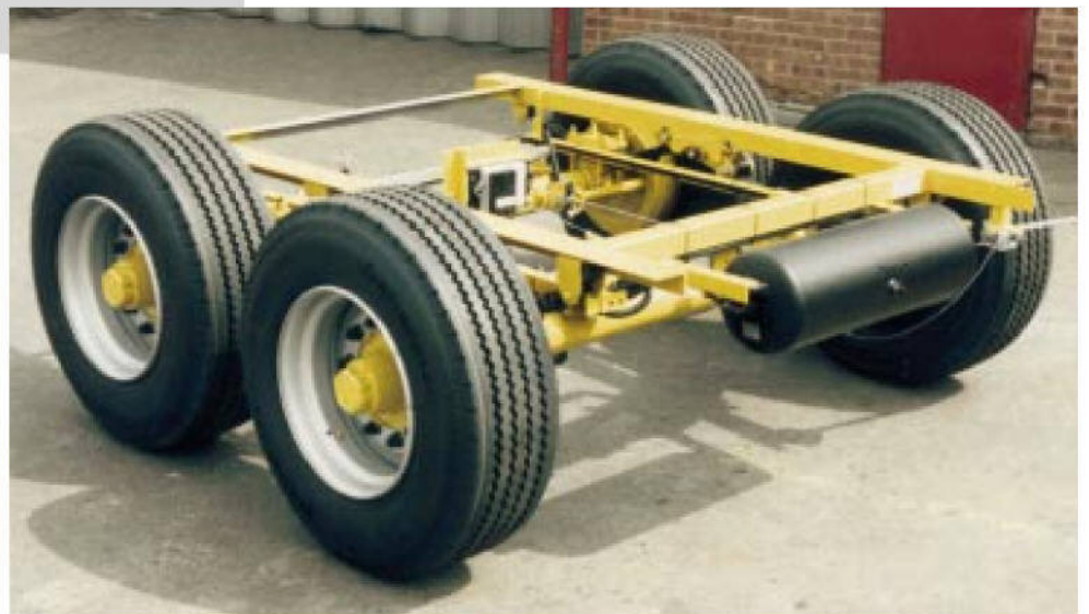
Lightweight bogie utilising the strength of the customer's chassis to allow a lighter and more economical construction
